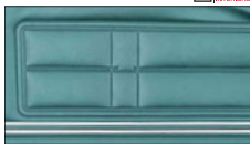
detail - dielectric pleats and twin chrome Mylar strips
