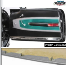
detail - door panel nail retainers are installed
