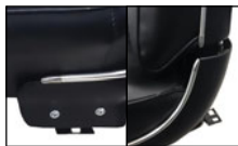
Most 1966-68 Side Panels Feature Correct Bullet End Caps
