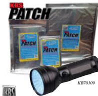
Cut KBS Patch into any size you want without exposing to UV or sunlight. Remove white backing tape to expose the sticky resin. Apply KBS Patch to repair area with sticky side down. Press firmly to repair surface. Remove transparent film backing and expose to sunlight or KBS UV Light. Curing times depend on UV intensity between 5 minutes (sunny) and 50 minutes (cloudy).
