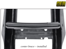
center brace - installed
