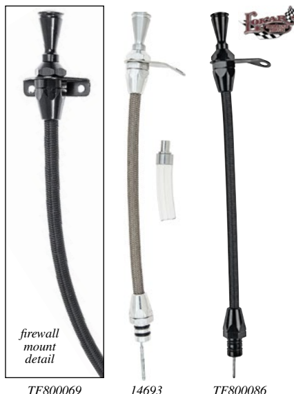
firewall mount detail
