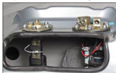
Fuel pump and sender are recessed in the tank for an easy installation.
