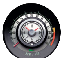
6468715 - red line at 6000 RPM with 7000 max RPM
