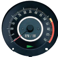
6468910 - red line at 5500 RPM with 7000 max RPM
