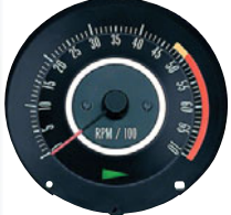
6468909 - red line at 5000 RPM with 7000 max RPM
