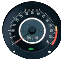
6468911 - red line at 6000 RPM with 7000 max RPM
